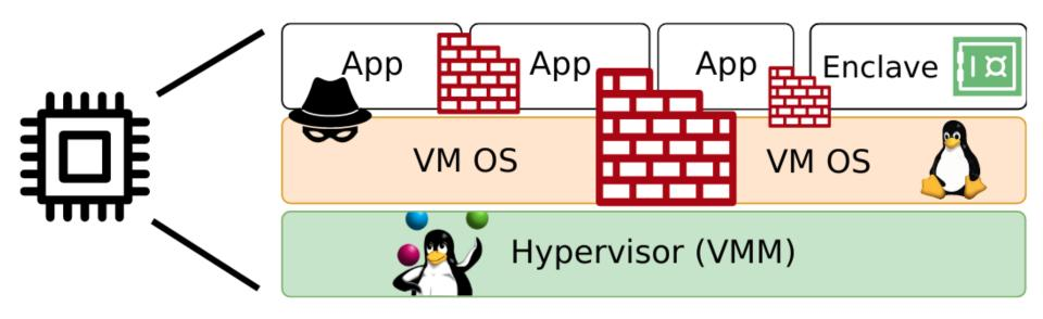
OS (and hypervisor, similar but not covered here) uses **CPU privilege rings** and **virtual memory** to build "walls" for memory isolation between applications
