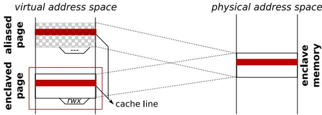
**Figure 6.4:** The physical enclave secret is mapped to an inaccessible virtual address for transient dereference.
