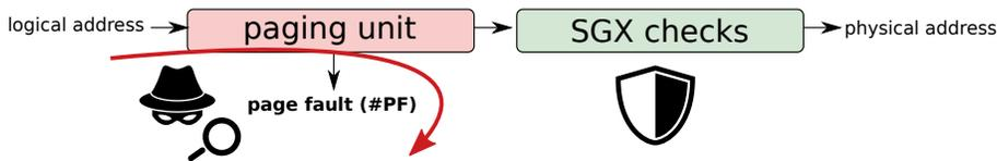
**Figure 8.1:** By provoking page faults in the untrusted address translation process, before SGX checks are applied, privileged adversaries can deterministically learn enclave memory accesses at a 4 KiB page-level granularity.
