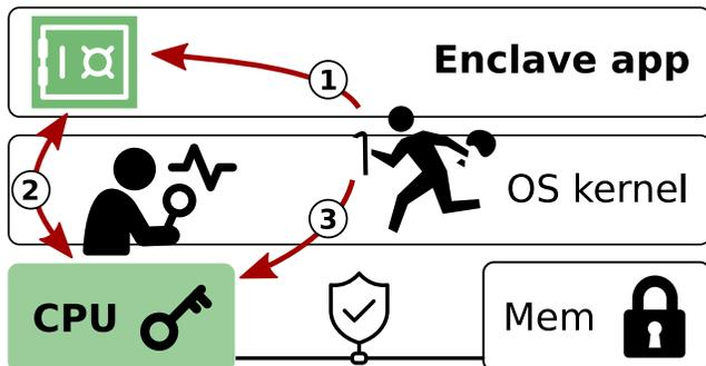
**Figure 1.5:** Three types of enclave interactions for privileged adversaries: (1) pass attacker-controlled arguments through the enclave interface; (2) derive execution metadata during or after enclave invocation through side channels; (3) extract enclave secrets from the CPU’s microarchitectural state through transient execution.
