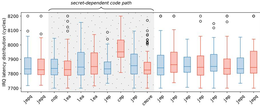
**Figure 5.11:** Interrupt latency distributions for 100 runs of Zigzagger branch taken (blue, left) vs. not-taken (red, right) execution paths.
