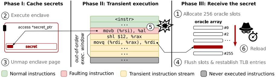
**Figure 6.2:** Basic overview of the Foreshadow attack to extract a single byte from an SGX enclave.
