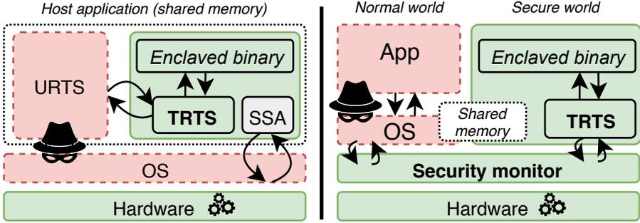
**Figure 2.1:** Enclave interactions in a single-address-space TEE design (left) vs. two-world design (right). The software components we study are bold, and the TCB is green (solid lines).
