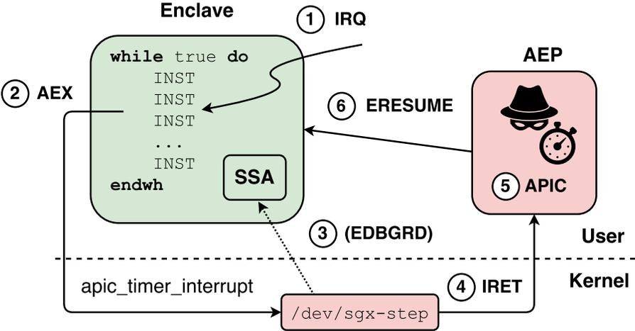
Figure 4.1: Framework for single-stepping SGX enclaves.
