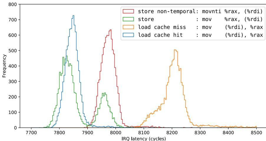
**Figure 5.9:** Increased interrupt latencies from enclaved data cache misses, from left to right: store, load hit, non-temporal store, load miss.
