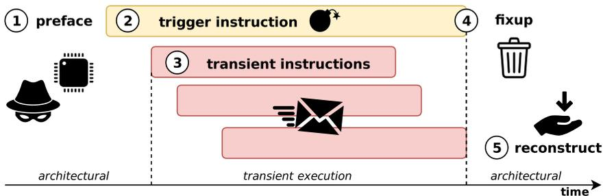
**Figure 1.4:** High-level overview of a transient-execution attack in 5 phases: (1) prepare microarchitecture, (2) execute a trigger instruction, (3) transient instructions encode unauthorized data through a microarchitectural covert channel, (4) CPU retires trigger instruction and flushes transient instructions, (5) reconstruct secret from microarchitectural state.
