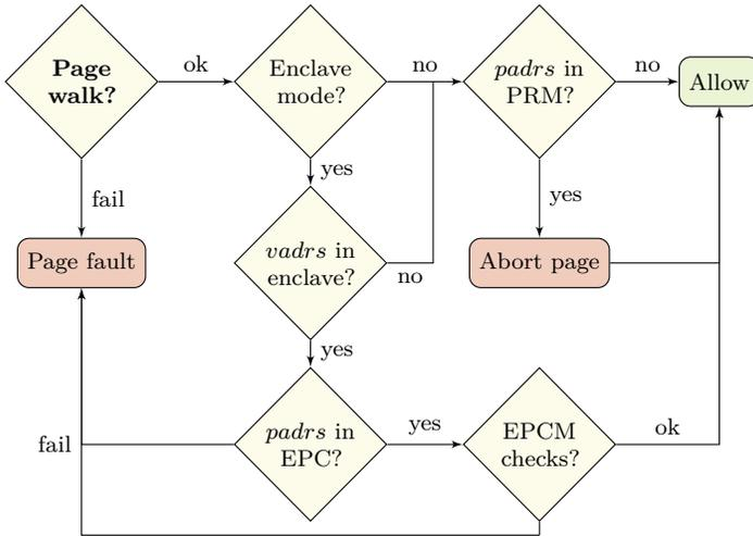
**Figure 3.1:** Additional memory access checks performed by SGX for a virtual address *vadr* that maps to a physical address *padr*.
