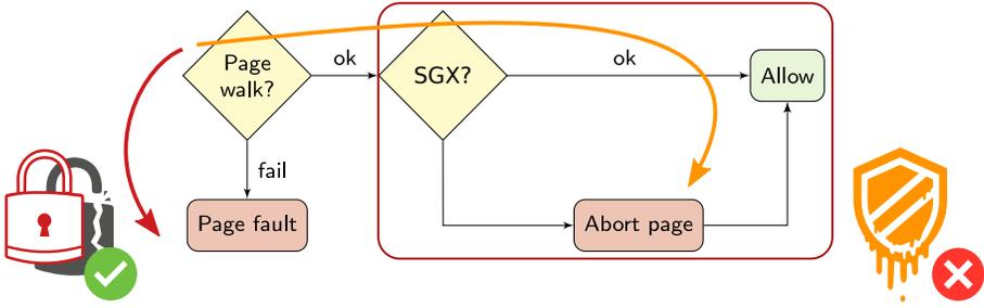
**Figure 6.3:** Naively applying Meltdown to transiently dereference SGX memory results in abort page semantics (right), whereas Foreshadow provokes a non-present fault in the untrusted page-table walk (left), before abort page semantics apply.
