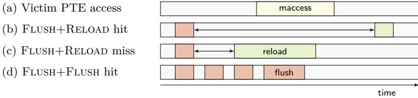
**Figure 3.3:** FLUSH+FLUSH as a high-resolution, low-latency channel to spy on victim PTE memory accesses.
