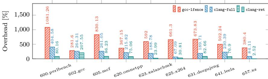
**Figure 7.10:** Performance overhead of Intel’s mitigations for non-optimized assembler gcc (fence loads + ret) and optimized clang (fence loads + indirect branch + ret vs. ret-only) for SPEC2017 on an Intel i9-9900K CPU.
