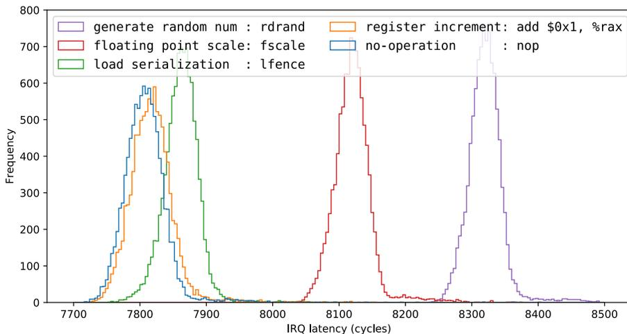
**Figure 5.7:** Interrupt latency distributions for selected x86 instructions, from left to right: `nop`, `add`, `lfence`, `fscale`, `rdrand`.
