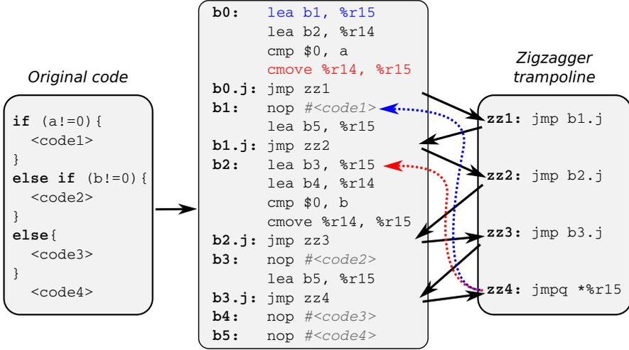
**Figure 4.2:** Example code snippet protected by Zigzagger. The final target address in `r15` is obfuscated with `cmov` and a tight trampoline sequence of `jmp` instructions (from [156]).
