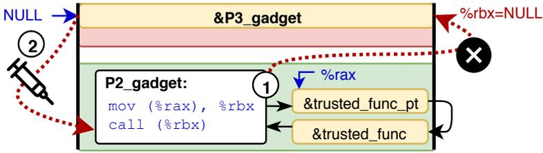
**Figure 7.6:** Transient control-flow hijacking using LVI-NULL: (1) a  $\mathcal{P}2$  gadget inside the enclave dereferences a function pointer-to-pointer, leading to a faulting load which forwards the dummy value null; (2) the following indirect call transiently dereferences the attacker-controlled null page outside the enclave, causing execution to continue at an attacker-chosen  $\mathcal{P}3$  gadget address.
