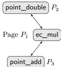
**Figure 3.2:** Code page layout for scalar point multiplication.
