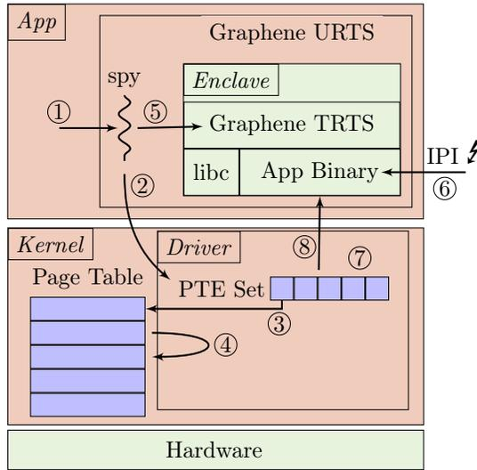
**Figure 3.4:** Graphene-SGX attack framework interaction.
