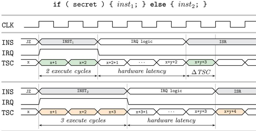
**Figure 5.2:** Interrupt latency leaks information about the instruction that was executing at the time of IRQ arrival.
