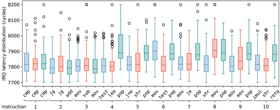
**Figure 5.12:** Interrupt latency distributions for 100 runs of `bsearch` left (blue) vs. right (red) vs. equal (green) execution paths.
