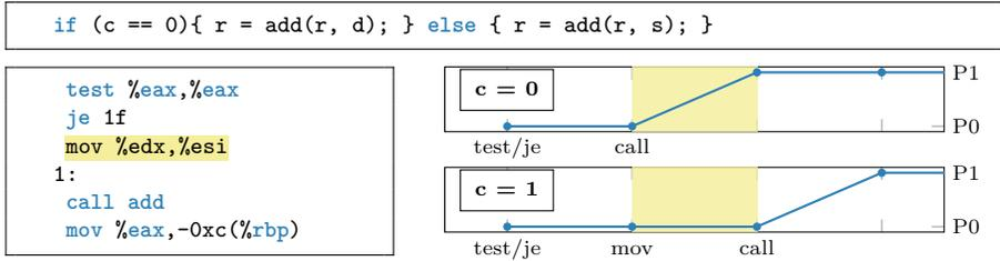
**Figure 8.2:** Balanced if/else statement (top), compiled to assembly (left). Precise page-aligned conditional control flow can be deterministically reconstructed with instruction-granular CopyCat page access traces (right).
