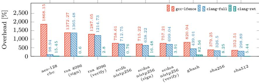
**Figure 7.9:** Performance overhead of Intel’s mitigations for non-optimized assembler `gcc` (fence loads + ret) and optimized `clang` (fence loads + indirect branch + ret vs. ret-only) for OpenSSL on an Intel i7-6700K CPU.
