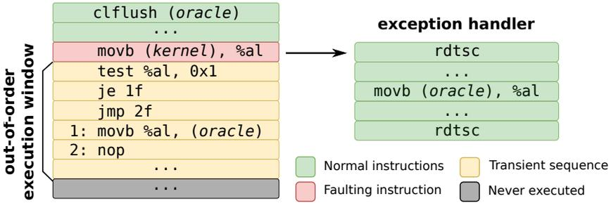
**Figure 6.1:** Rogue data cache loads can be leveraged to leak sensitive data from more privileged security layers.
