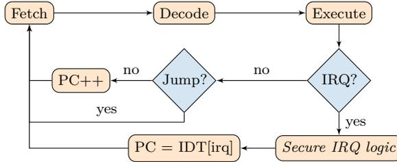
**Figure 5.1:** A processor fetches, decodes, and executes the instruction referred by the Program Counter (PC) register.
