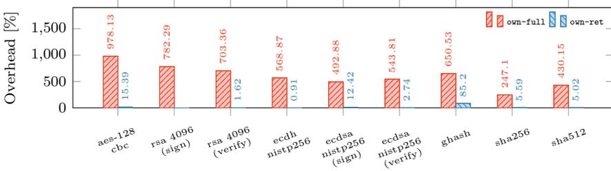
**Figure 7.8:** Performance overhead of our LLVM-based prototype (fence loads + ret vs. ret-only) for OpenSSL on an Intel i7-6700K CPU.
