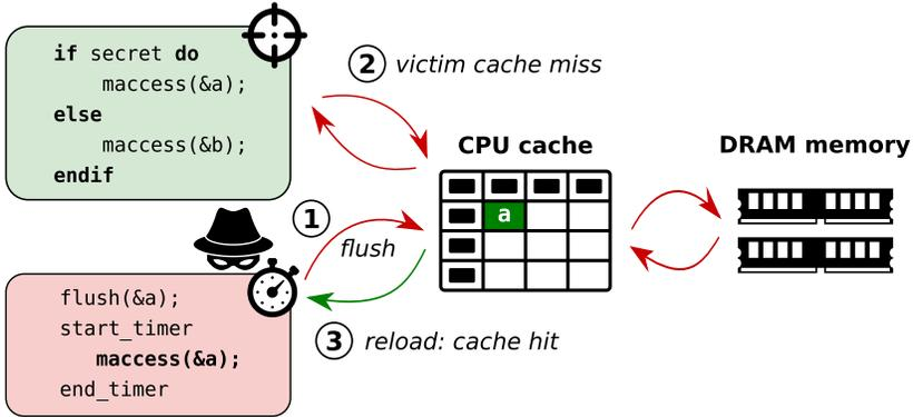
**Figure 1.3:** Overview of a FLUSH+RELOAD side-channel attack to learn whether a victim program accessed a shared memory region in three phases: (1) the attacker flushes the shared memory region from the CPU cache; (2) the victim program conditionally accesses the shared memory region, depending on some secret; (3) the attacker learns whether the victim brought the shared memory location into the CPU cache by measuring the amount of time it takes to reload that location.
