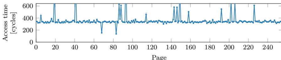
**Figure 7.4:** Access times to the probing array after the execution of Listing 7.1. The dip at 68 (‘D’) is the transmission specified by the victim’s architectural program semantics. The dip at 83 (‘S’) is the victim secret at the address `untrusted_arg` injected by the attacker.
