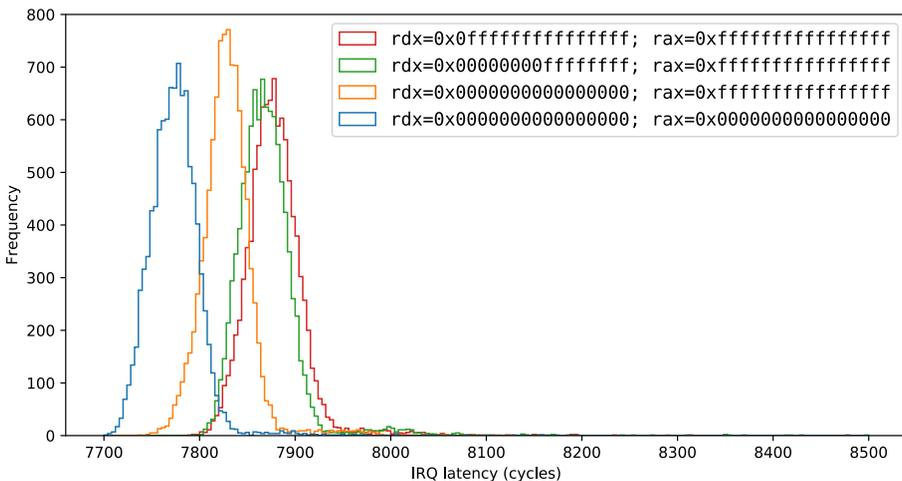
**Figure 5.8:** Data-dependent interrupt latencies for the x86 `div` instruction with from left to right an increasing amount of bits set in the dividend operand.
