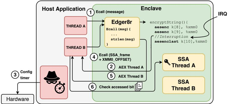
**Figure 2.4:** Overview of the key extraction attack exploiting `strlen()` side-channel leakage in Intel SGX SDK.
