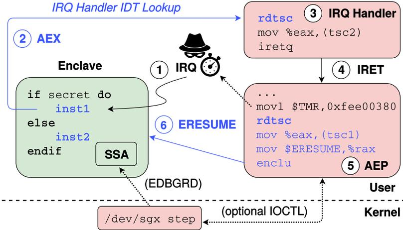
**Figure 5.5:** Enhanced SGX-Step framework for precise interrupt latency measurements (blue path) on Intel x86 platforms.
