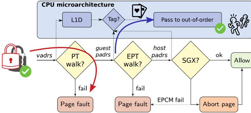
**Figure 6.9:** CPU address translation and L1 terminal fault behavior: documented architectural view (bottom) and undocumented microarchitectural transient-execution interactions (top).
