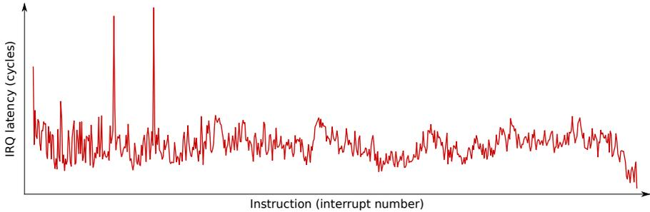
**Figure 5.4:** Sample interrupt latency trace revealing execution timings for individual SGX enclave instructions.
