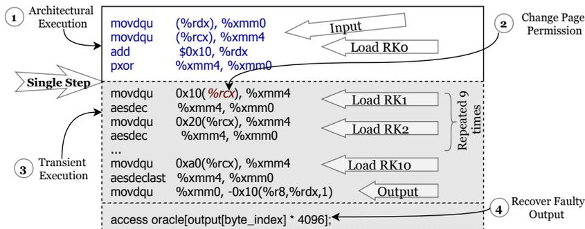
**Figure 7.7:** Overview of the AES-NI fault attack: (1) the victim architecturally executes the initial AES round, which `xors` the input with round key 0; (2) access rights on the memory page holding the key schedule are revoked; (3) upon the next key access ( $P2$ ), the enclave suffers a page fault, causing the CPU to transiently execute the next 10 AES rounds with zeroed round keys; (4) finally the faulty output is encoded ( $P3$ ) through a cache-based side channel.
