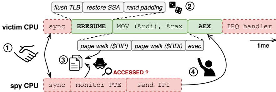
**Figure 8.3:** Adversaries can precisely single-step a victim enclaved execution (green, solid) without resorting to timers by sending inter-processor interrupts from a concurrent spy thread (red, dashed) that monitors unprotected page-table accesses.
