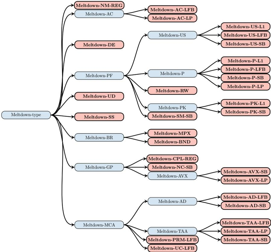
**Figure A.1:** State-of-the-art classification tree for Meltdown-type attacks [36].
