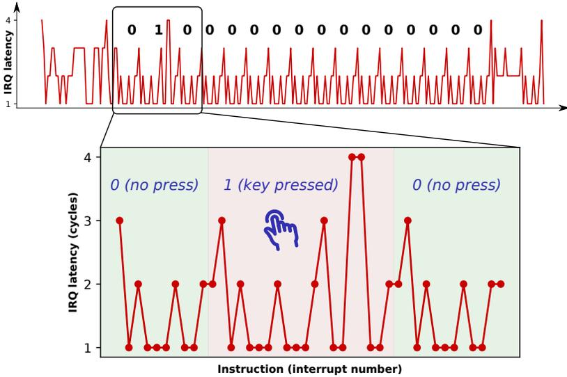
**Figure 5.6:** Interrupt latency trace revealing keystrokes in a Sancus enclave.
