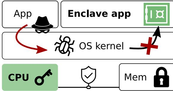
**Figure 1.2:** Trusted execution environments, like Intel SGX, offer hardware-level isolation and attestation for unprivileged software components, called *enclaves*, using a cryptographic key that never leaves the CPU package. The processor furthermore prevents unauthorized accesses to enclave-private memory by *any* outside software, including traditionally privileged operating system or hypervisor layers.
