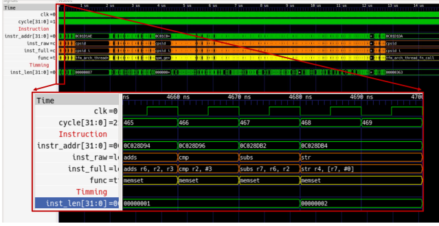
Figure 8: Example of the Mstp-Visualizer depicting the PoC trace of the standard printf function from stdio.h .
